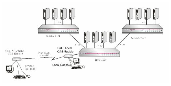
Figure 17 Two-Tier Configuration (with optional Remote Access Kit)
